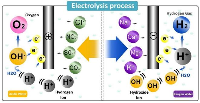
**STEP 2: ELECTROLYSIS** through several\* electrode plates and membranes, the filtered water is separated into acidic and alkaline parts. Water is spited into OH-(hydroxide ions) and H+ (hydrogen ions).
